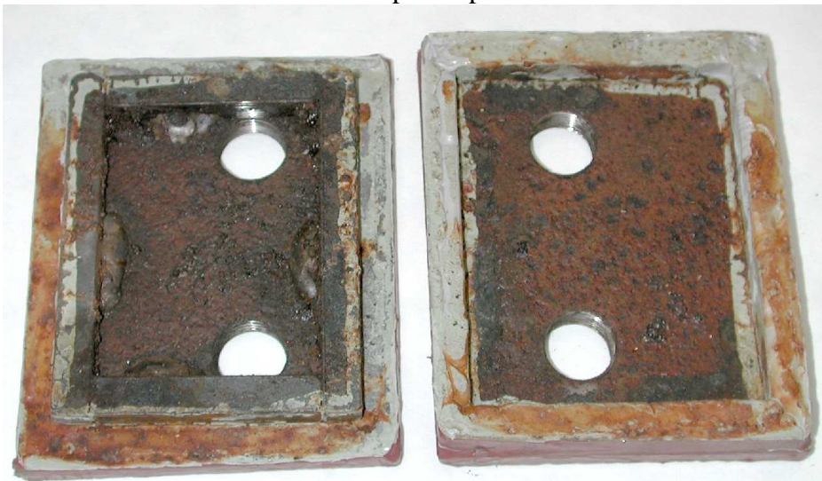
RPCS 8 - Rusting of interface of cement and steel
