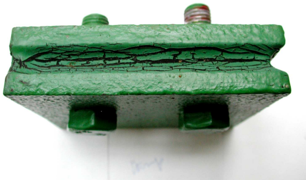
RPCS 10 - cracks in paint and cement
