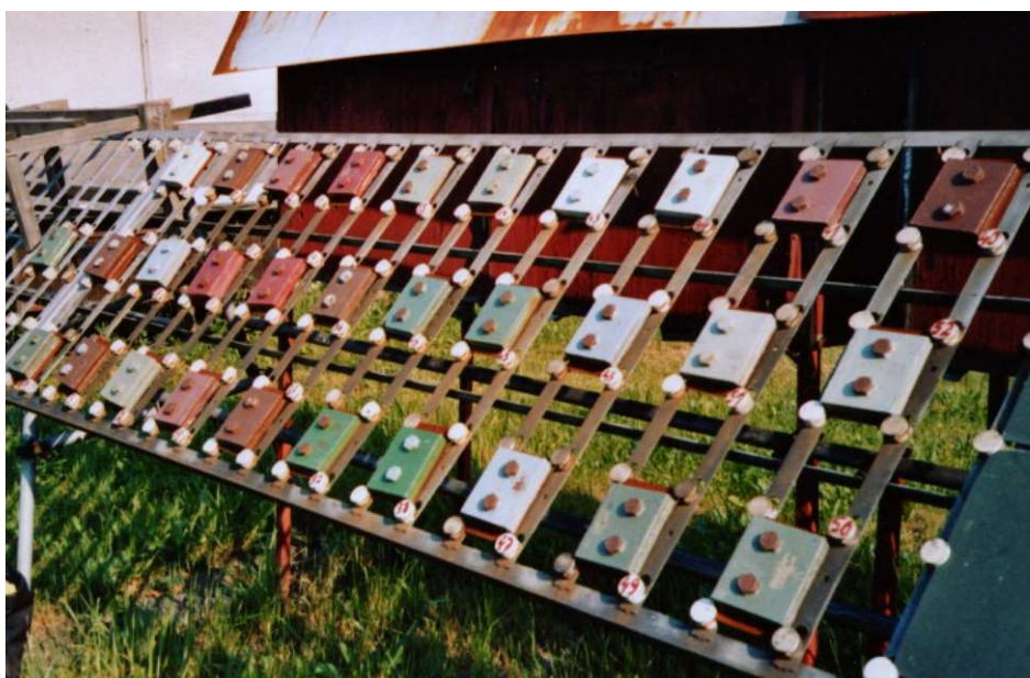
Figure 5 - Exposure of samples with model crevice at atmospheric test site
