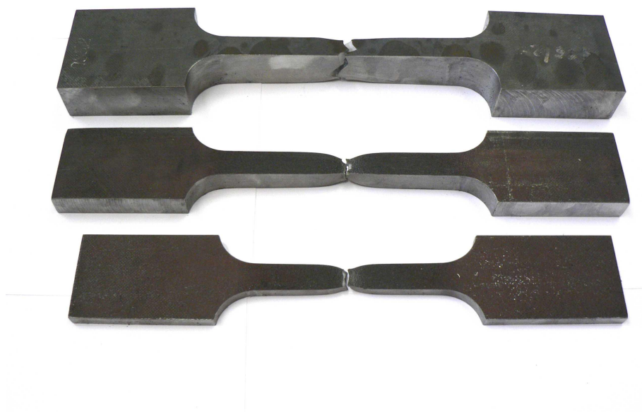
Fig. 4. Tension tests flat samples with thickness 10, 20 and 35 mm after fracture
